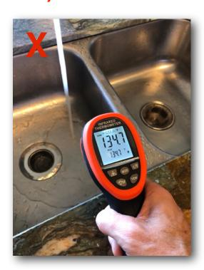
The hot water temperature at the kitchen sink is 134°F. This is considered hazardous - contact for 15 seconds can produce a 3rd degree burn. Children and elderly are especially sensitive to this. The safety standard for scald prevention is a maximum 120°F. The temperature was not checked at other fixtures to determine if they incorporated updated anti-scald fixtures.
